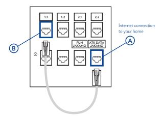
**Tip:** If you do not know which socket in the distribution box connects your home to the Internet, you can identify the correct socket by connecting your computer directly to the distribution box via a cable and by testing which socket is connected to the Internet.
